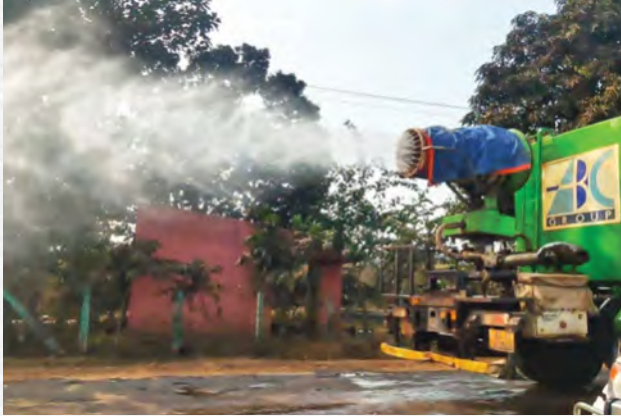
Truck Mounted Fog Cannon (40 m throw) deployed at Lakhanpur OCP
